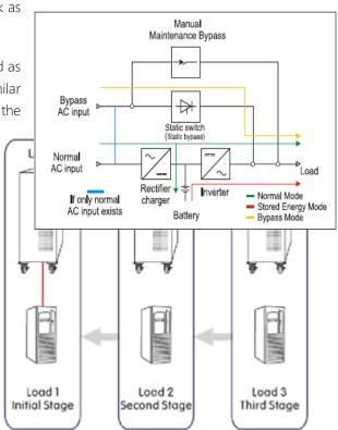
Parallel Expansion Schematic Diagram
