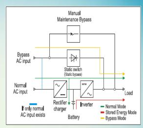
clean and protected power free of site voltage and frequency fluctuation. Your equipment always receive a stabilized power thru the UPS Inverter and built-in AVR function. The REL2900PRO-33 provides backup power thru built-in batteries and keeps your critical load protected at all times. The battery autonomy time can be increased to any duration by installing External Battery Banks.
